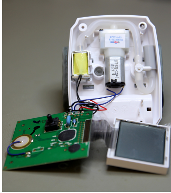
Figure 3: Internals of blood pressure monitor before disassembly.
