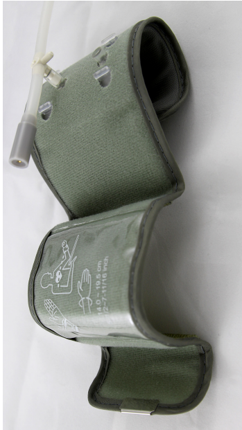
Figure 2: Users only wear the bare wristband from the blood pressure monitor on their arm. All electronic components are moved to an external controller.
